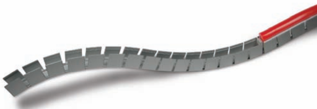
Vertical Notched Channel TVFP-NOTCHV-6.5 Concave bend to 6" minimum radius Convex bend to 4" minimum radius
