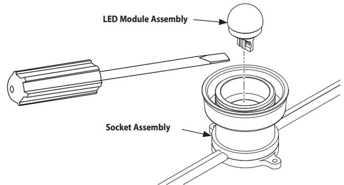
**Step 3:** Install replacement LED Module by inserting gently into socket until it locks into place.
