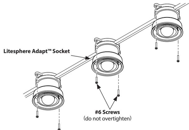
**Step 3:** Litesphere Adapt is manufactured with a 24" Lead Wire at both ends in order to ensure the globes will be mounted at least one foot away from any structure. However, for rigid mounting, the dead end lead may be cut back in the field to 1 1/16" minimum, which is just long enough to fit inside the End Cap (LS-EC-CL, included). For best results, fill the inside of the End Cap with Silicone Sealer before installing on wire.
