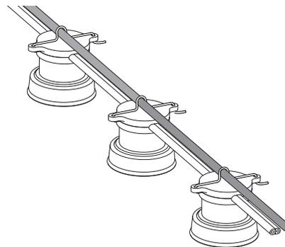
**Step 13:** Litesphere Adapt is manufactured with a 24" Lead Wire at both ends in order to ensure the globes will be mounted at least one foot away from any structure to avoid damage to a globe if it comes in contact with the structure. If strand is trimmed in the field, be sure to maintain the 24" lead at the end of the strand. Install an End Cap on the trail end (LS-EC-CL, included). For best results, fill the inside of the End Cap with Silicone Sealer before installing on wire.
